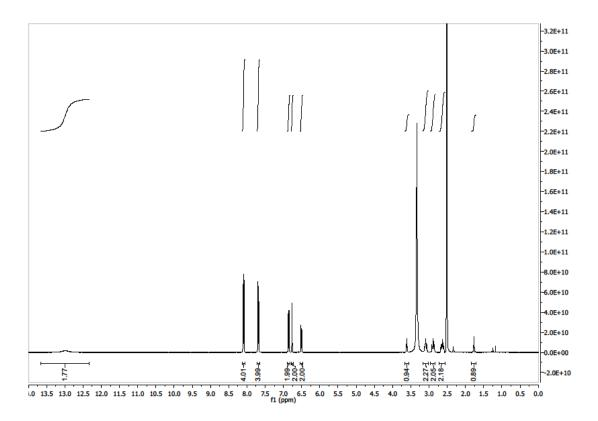
Figure 1 – The <sup>1</sup>H-NMR spectrum of pp-bis(4-carboxyphenyl)[2.2]PC, recorded in DMSO-d6.
