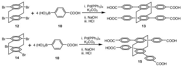
Scheme 4 – The synthesis of the two desired tetracarboxylated linkers.
